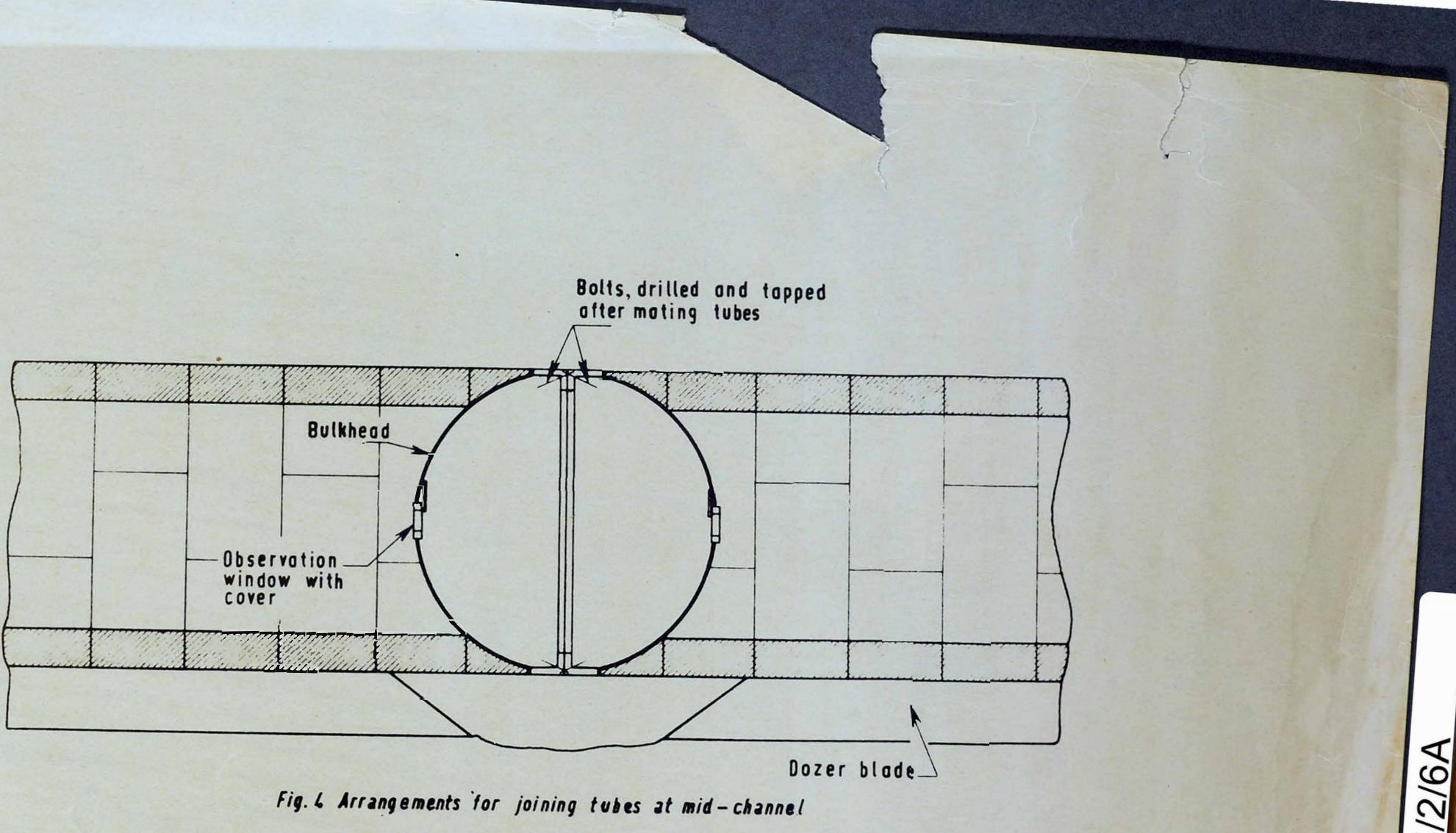
Fig. L Arrangements for joining tubes at mid-channel
